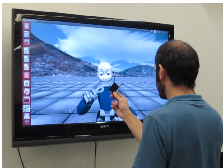
Figure 7. The experimental setup: Avatar is displayed on a big screen (46 inches; Sony KDL-46V4000). The iCub robot (in the simulator) is leading and the participant is following the motion. The participant holds a marker for recording purposes.
